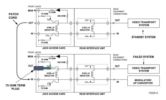
Figure 30. Bypass Failed Video System
